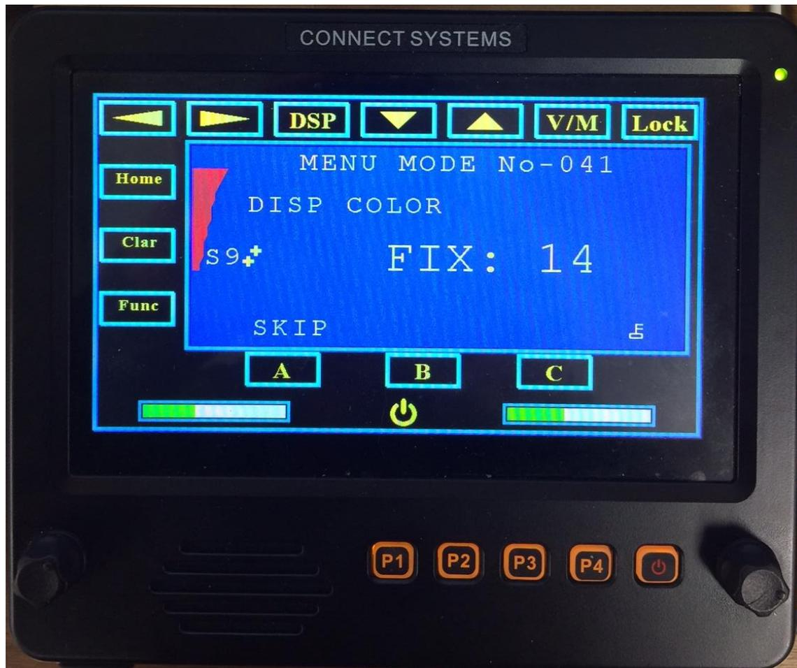
The knob on the right is used for the volume control and the knob on the left is used for squelch control. Once you set levels the way you want them, press the P1 switch again to get out of that mode.
