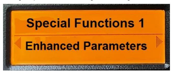
If the voice was enabled, then it would annunciate "Special Functions 1 Enhanced Parameters". If this screen appeared as the result of pressing P5 or P6, then it would annunciate "Enhanced Parameters"
