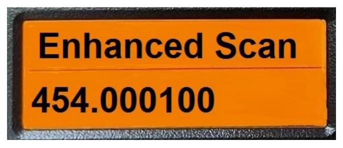
Now the program is looking for the GPS module so it can determine the nearby repeaters so it can make a correction to its transmitter frequency if necessary.
