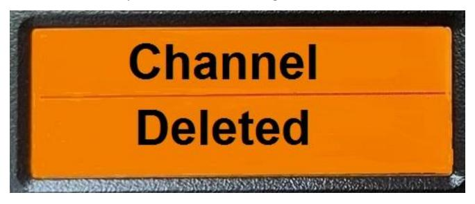
If the voice prompts are enabled, then the radio will annunciate Channel Deleted.
