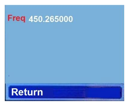
The Frequency parameter is always a nine-digit number. The program puts a decimal point after the first three digits. The first digit must always be a 4 or a 5. If the user puts in something else, the program will put in a 4.
