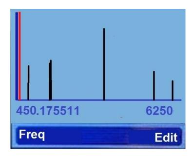
The frequency value on the display corresponds to the red cursor. To move the cursor to the right, press the up-arrow key. To move the cursor to the left, press the down-arrow key.
