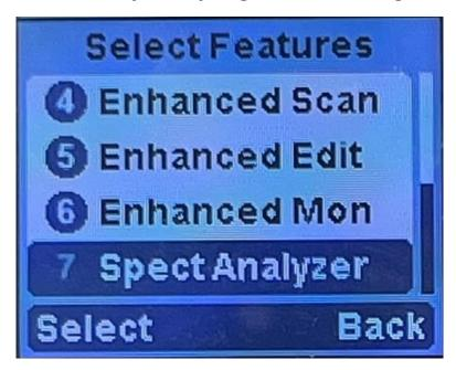
Press the OK key and you start the Spectrum Analyzer program as shown in the rest of this application note.
