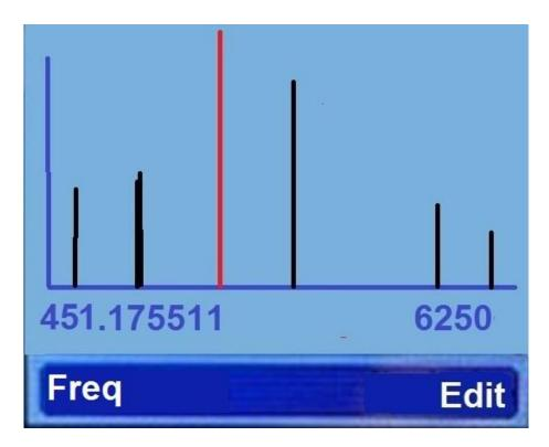
Pressing the "1" key will decrease the offset for the noise on the display. Pressing the "3" key will increase the offset for the noise on
