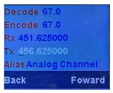
The Tx Frequency parameter is always a nine-digit number. The program puts a decimal point after the first three digits. The first digit must always be a 4 or a 5. If the user puts in something else, the program will put in a 4.
