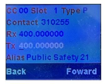
The Tx Frequency parameter is always a nine-digit number. The program puts a decimal point after the first three digits. The first digit must always be a 4 or a 5. If the user puts in something else, the program will put in a 4.
