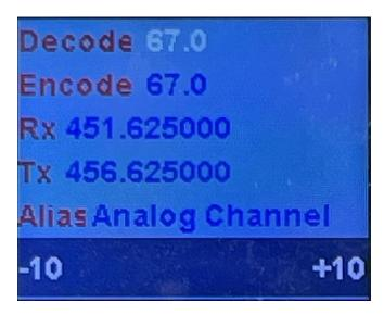
The Decode parameter is arranged as a table. The first 50 entries in the table is CTCSS. The next 104 entries is the DCS code and the last 104 entries is the inverted DCS codes.
