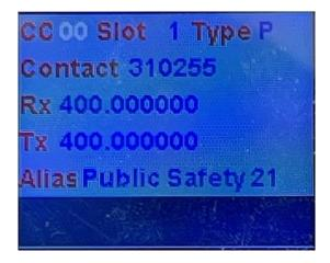
The Color Code parameter is arranged as a table with values of 00 to 15.
