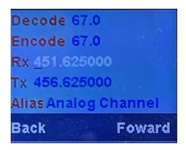
The Rx Frequency parameter is always a nine-digit number. The program puts a decimal point after the first three digits. The first digit must always be a 4 or a 5. If the user puts in something else, the program will put in a 4.
