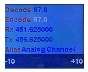
The Encode parameter is arranged as a table. The first 50 entries in the table is CTCSS. The next 104 entries is the DCS code and the last 104 entries is the inverted DCS codes.
