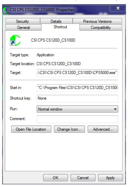
Modify the Target: Line by adding -K at the end as follows:
