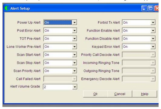
Each alert can be individually programmed as ON or OFF. On mean the feature will be valid. OFF mean the feature will be invalid.
