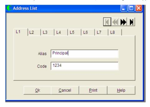
This screen allows the entry of telephone numbers. The user should enter the name of the telephone (alias) and the telephone number (code).
