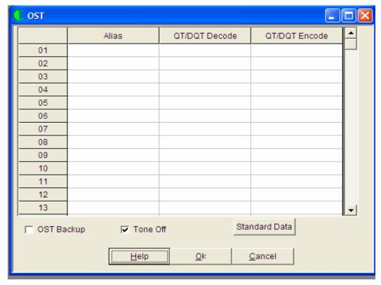
The OST screen allows the radio user to dynamically assign the CTCSS and DCS decode and encode values on the selected channel by pre-programming the table.
