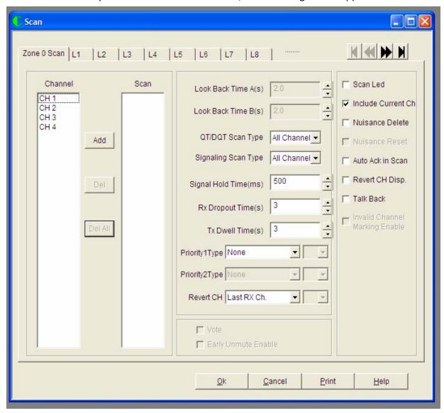
This menu is used to set the feature of scan. There 17 scan list available. Zone 0 Scan list can be used to scan all channels in the system. Zone 1 – Zone 16 Scan list can be used for scanning only 16 channels each.
