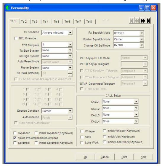
The personal template is used in the Channel Edit menu to allow the dealer to set groups of channels with the same property. Up to 16 different personal templates can be set up.
