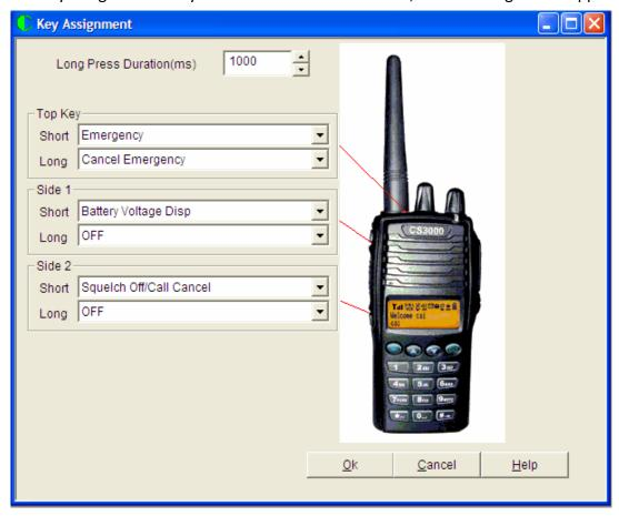
There are three buttons on the radio that are programmable for different functions. Each button has the capability of having two separate functions, determined by how long the button is pressed. The length of time the button has to be pressed for the second feature is determined by the dealer. The list below gives the possible features and the reasons for the features. The user must be informed by the dealer the function of each key.
