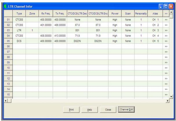
This screen is a summary of the Channel Information. To set the parameters for the channel press the Channel Edit key and access the screen shown on the next page.
