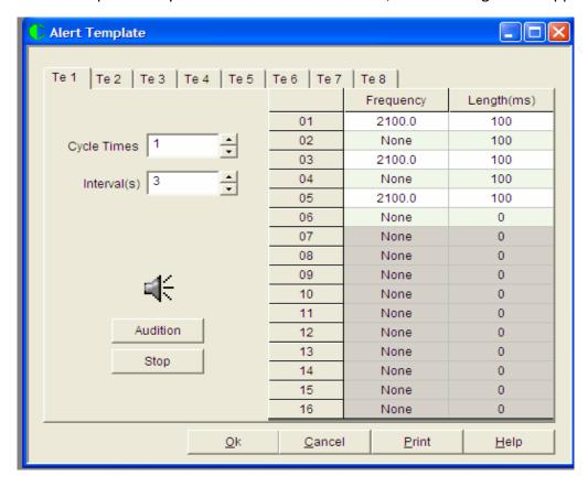
Alerts are used for detecting incoming signaling. Up to 16 different alerts can be programmed in this system. Each alert can consist of up to 16 different tones. These alerts are used in the following screens:
